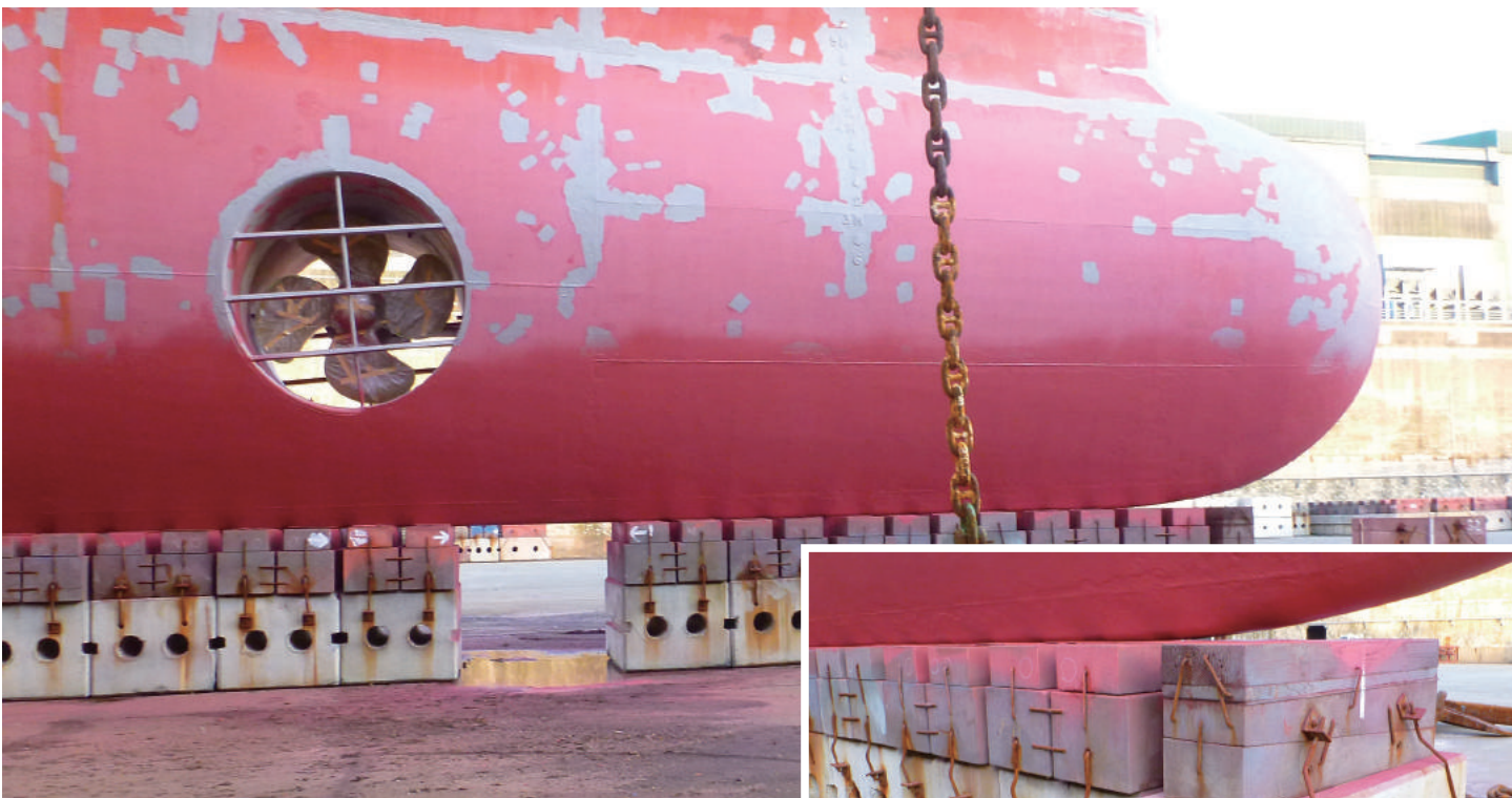
塗料が柔らかいが人工盤木が柔らかいため 船底塗料に対しダメージが少ない The paint is soft, but bottom paint damage is small because Artificial wood board is soft.
