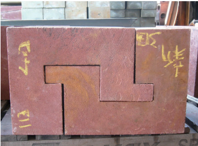
追い掛け継手 継手部長尺盤木時には途中に継手を入れて製作します When I produce a long Artificial wood board on joints, I put the joint in the middle.
